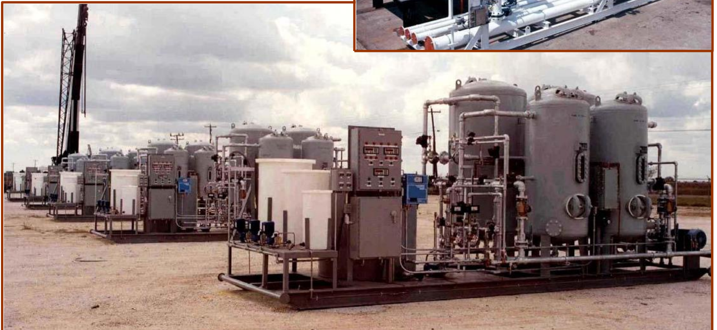
Sets of Tecnolog Dual Bank Water Softener and Chemical Feed Systems for APIN™ Oil Field Steam Generators.
